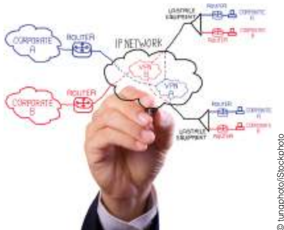
FIGURE 4.2 Virtual private networks (VPNs) create encrypted connections to company networks.
